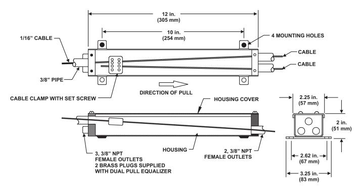
Note: Use 3/32 in. hex key for cable pulley set screws.
